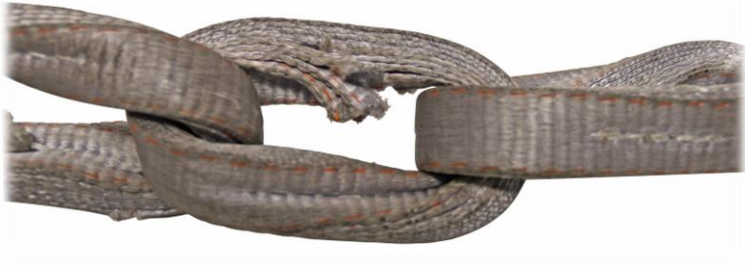
Fig. 1: Cut webbing layer inside.
