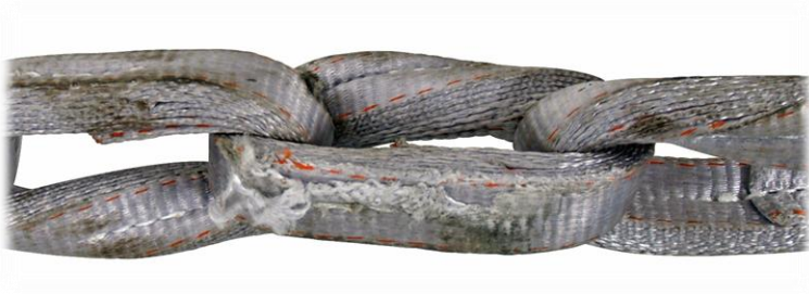
Fig. 3: Abrasion on the surface of the chain link
