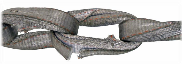
Fig. 2: Cut webbing layer outside.
