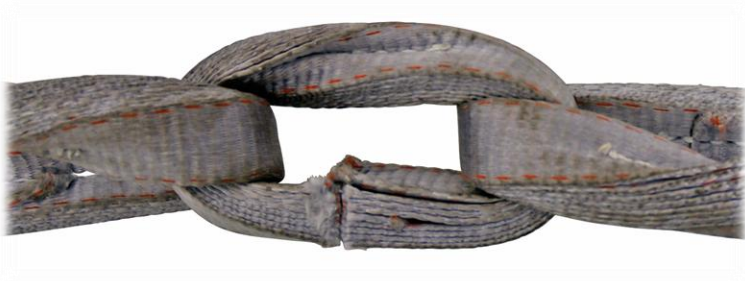
Fig. 4: cut in the chain link
