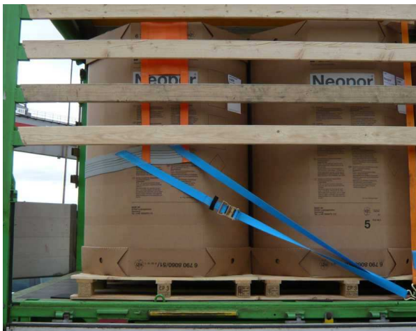
pic. 10: example for securing Oktatainer with the DoUniFlex-securing system (extended)
