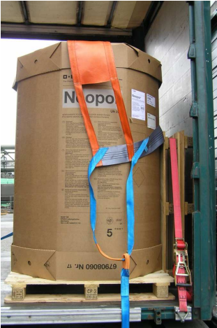
Pic. 6: position the DoUniFlex-securingsystem on the load (shown: Oktatainer®)
