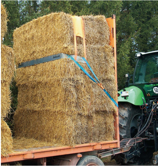
pic. 12: example for securing straw bales with the DoUniFlex-securingsystem standard.
