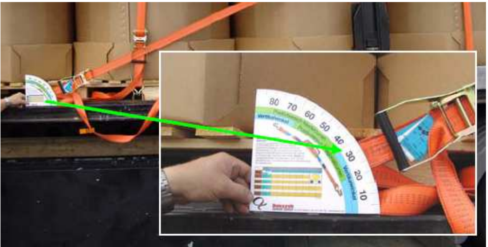
Pic. 8: Consideration of lashing angle \alpha of approx. 30^\circ
