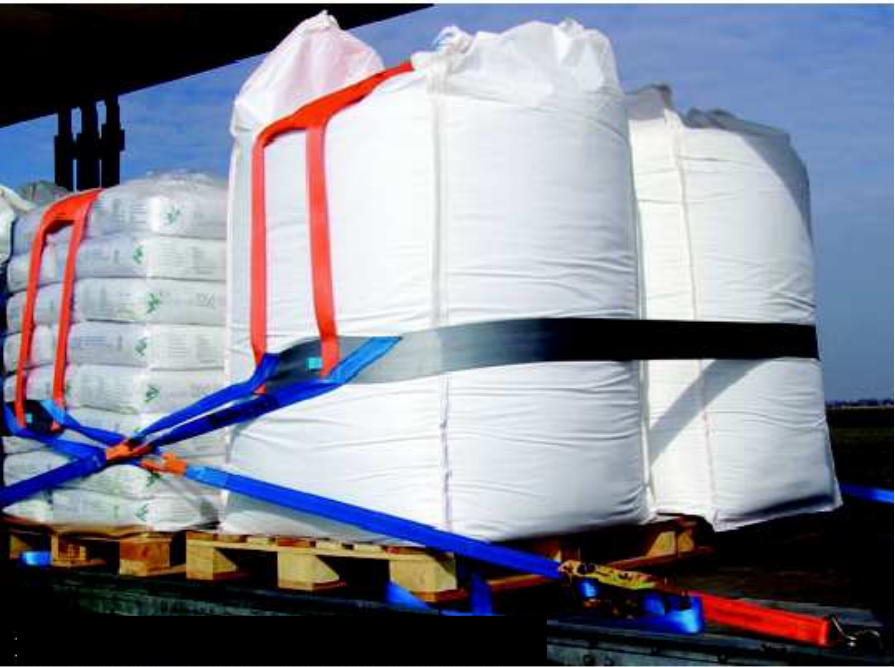
pic. 11: example for securing BagBags and bagged goods with the DoUniFlex-securing system (standard)
