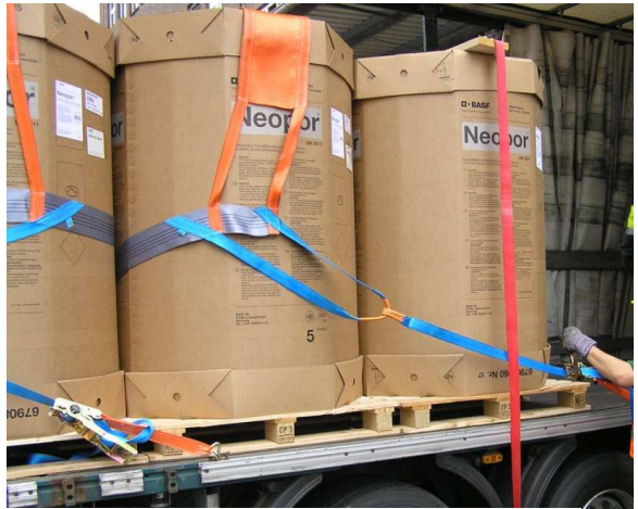
pic. 7: connect the loose-end of the DoUniFlex-securingsystem with a short part of a standard lashing strap. Make sure that the Lashing-angle is approx 30^\circ
